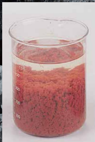
絮凝后的污泥状态 Sludge state after flocculation
