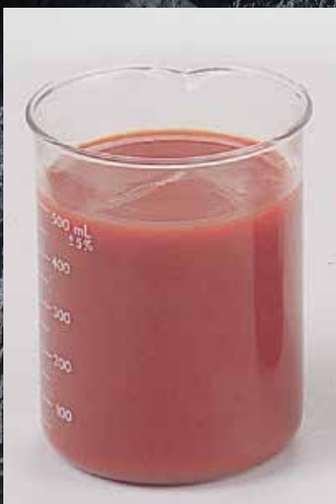
脱水前的污泥水 Sludge water before dewatering
