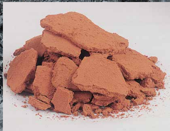
脱水后的泥饼 Sludge cake after dewatering
